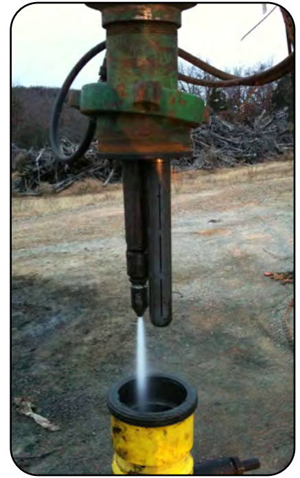
Function testing jetting tool on surface prior to running in hole.
